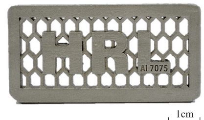
图10 SLM成形的7075合金HRL标志 Fig.10 7075 alloy HRL logo fabricated by SLM
